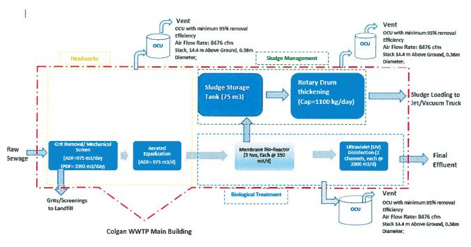
Figure 3. Process Flow Diagram, Colgan WWTP
