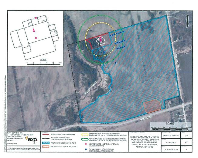
Figure 1. Site Plan, Colgan Wastewater Treatment Plant – emission source location and, existing and future receptors
