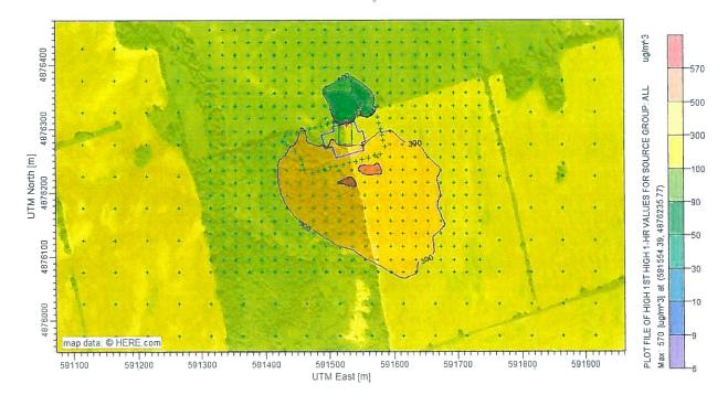
Figure 6. AERMOD modelling contours- emergency generator emissions
