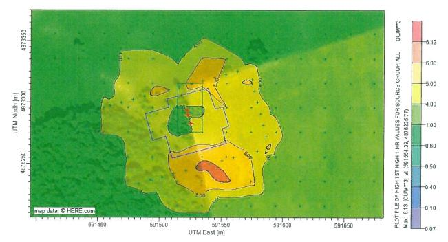
Figure 5. AERMOD modelling contours- process emissions
